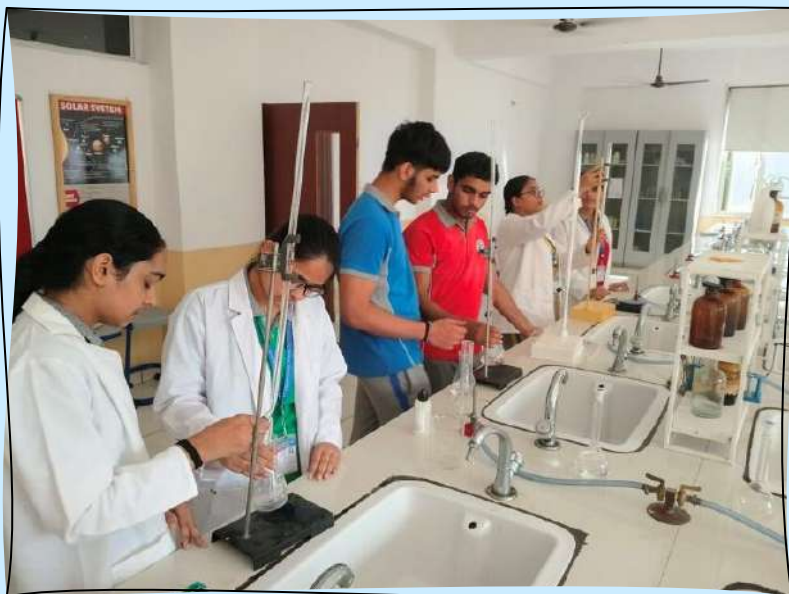
Recording the burette reading at the point of neutralisation
