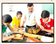
The Wheatstone bridge is a fundamental circuit used to measure unknown electrical resistances. It operates on the principle of balancing two legs of a bridge circuit. When the bridge is balanced, the ratio of the resistances in one leg is equal to the ratio of the resistances in the other leg, allowing for precise
